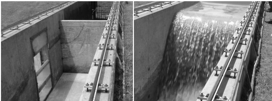
Figure 3.3 Depiction of Floodwall Testing
